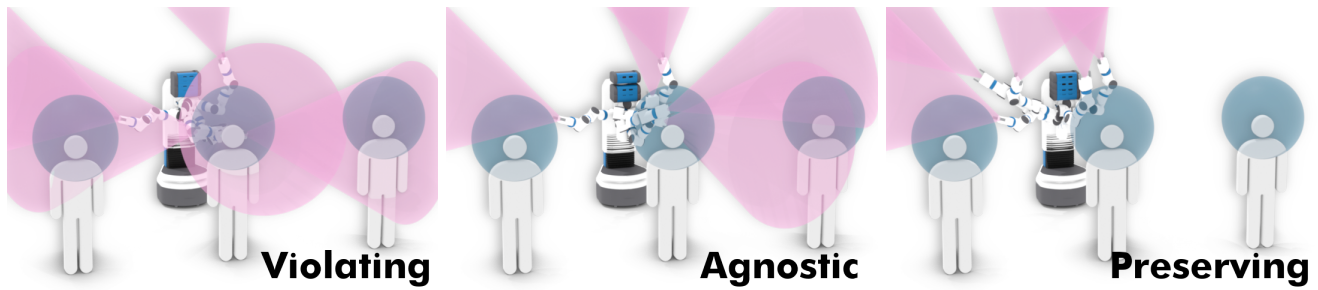
Fig. 4. The visualization of different privacy-aware behavior: violating (left), agnostic (middle), and preserving (right) showing snapshots of the pink camera cone along motions solving the same problem. Even the agnostic path sweeps the camera cone over the right privacy region. The violating path makes the camera cone intersect with all the privacy regions while the preserving one avoids them altogether.
